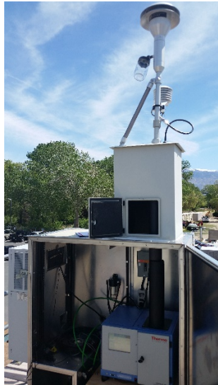
Photographs 1 and 2. PM10 Air Monitoring Equipment Platform and Location
